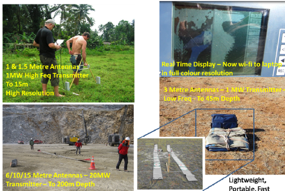
Figure 1: Terravision Radar equipment. The Radar is configured as follows:
