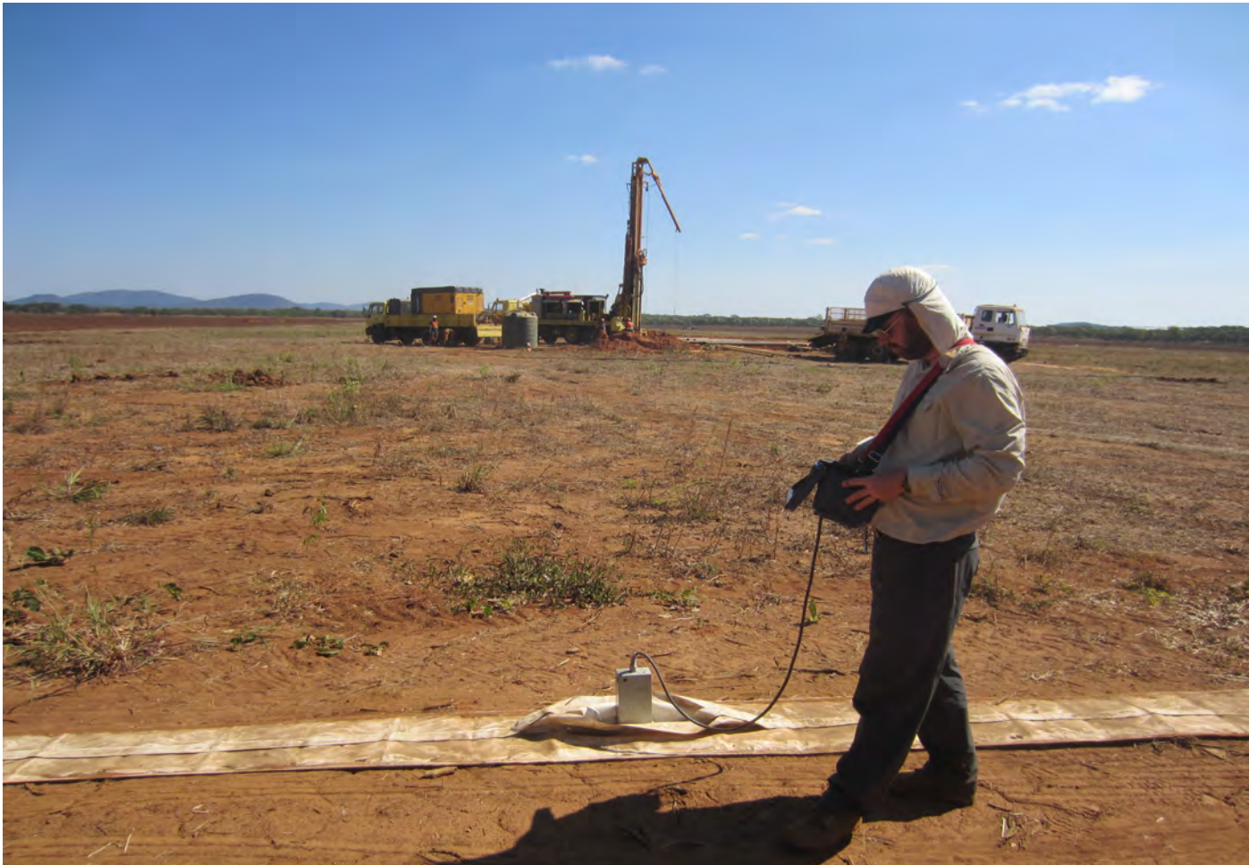
Left: the image shows the radar in action, close to a drill rig whilst surveying for intrusives in Botswana 2014.
