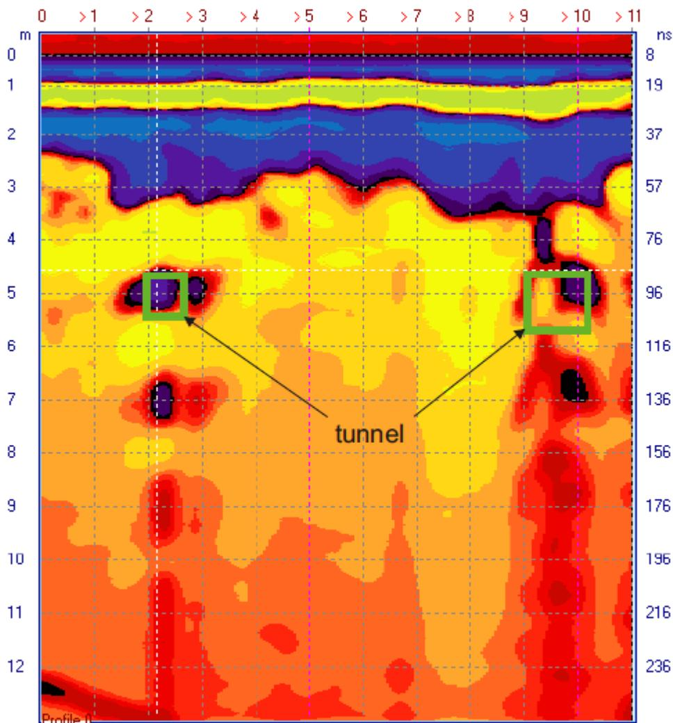
Fig 12. Radargram showing identified voids in the limestone.
