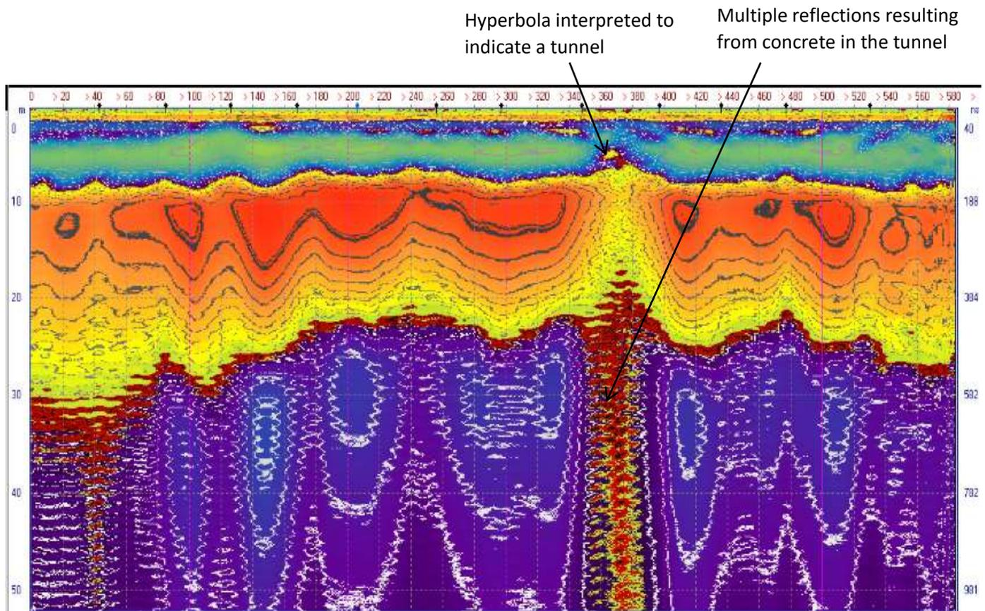
Fig 7. Radargram showing a void at 5 m depth interpreted as an old mine working.
