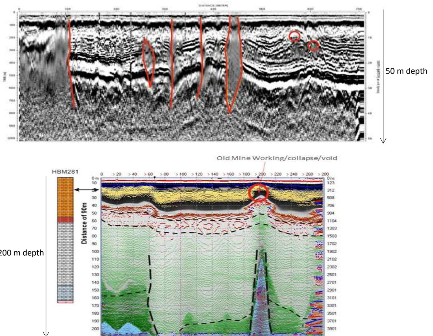
Fig. 10: Above Radargram shows Terravision data using REFLEX software to 50 m depth. The lower Radargram shows data from a different profile line in the Terravision software krot to 200 m depth
