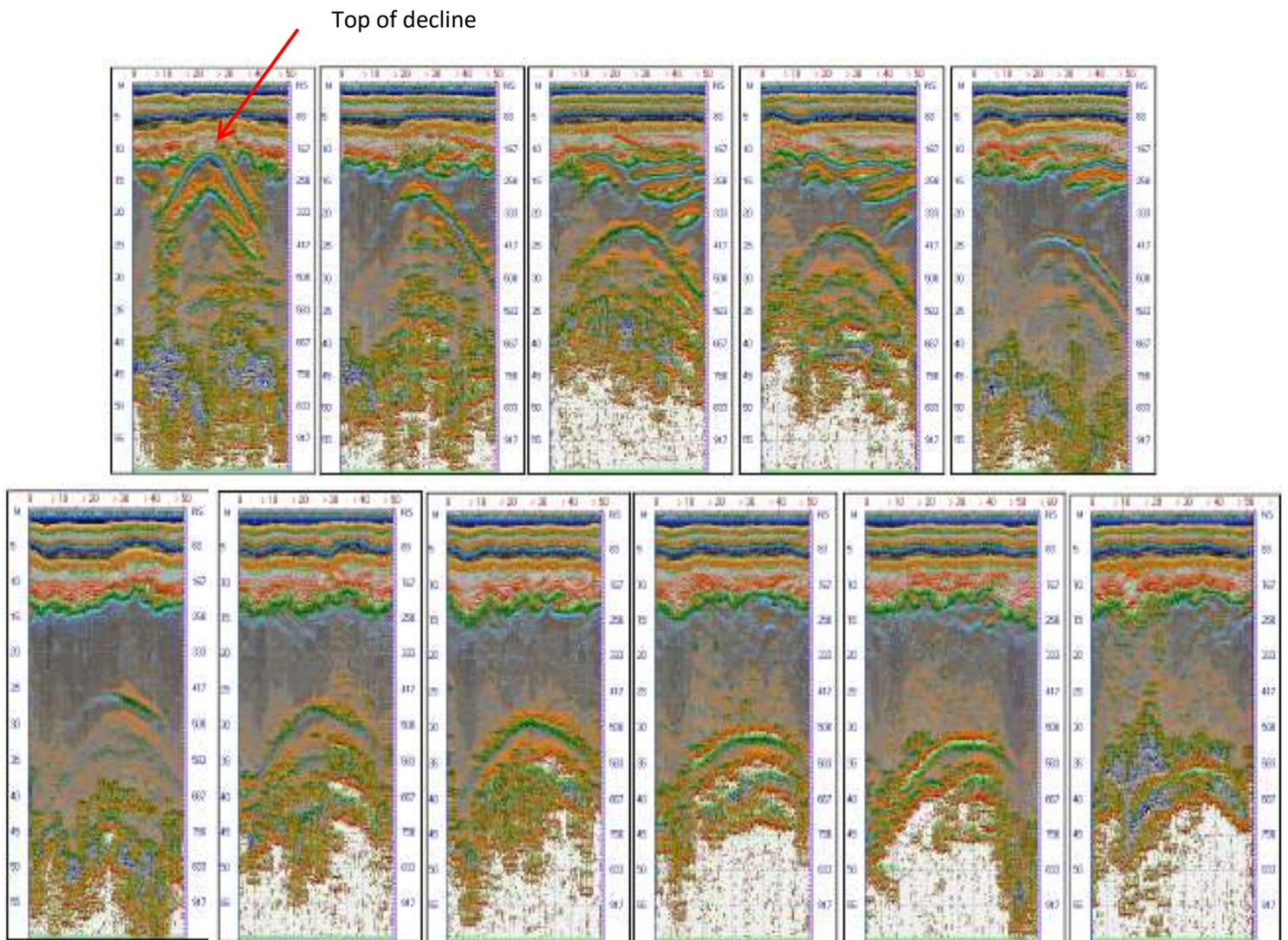
Fig 9. Radargrams taken at 10 m spacing showing the decline of a mine shaft.
