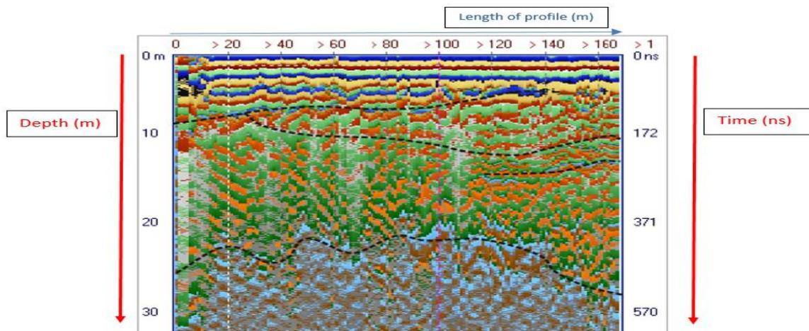
**Fig 3. Radargram illustrating scales**
