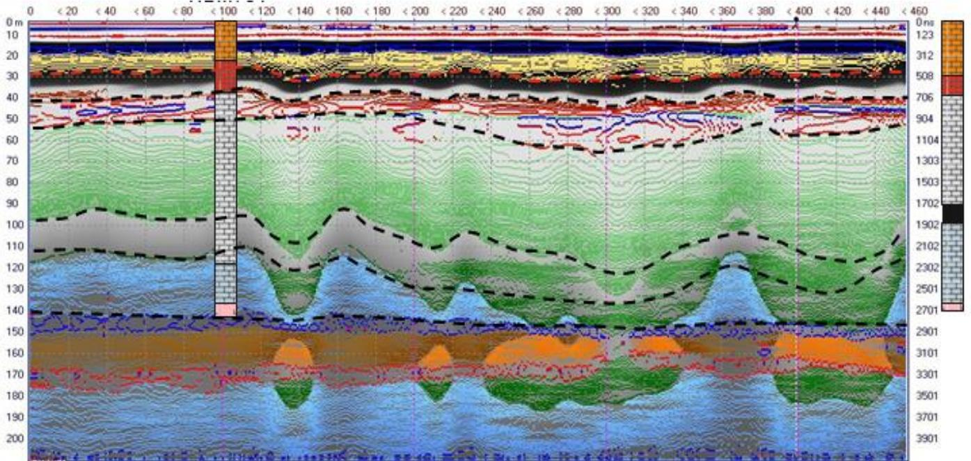
**Fig 6. LF Radargram with borehole lithology overlaid.**
