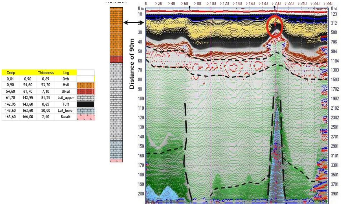
Fig 8. LF data with borehole correlation and showing a vertical karstic feature.
