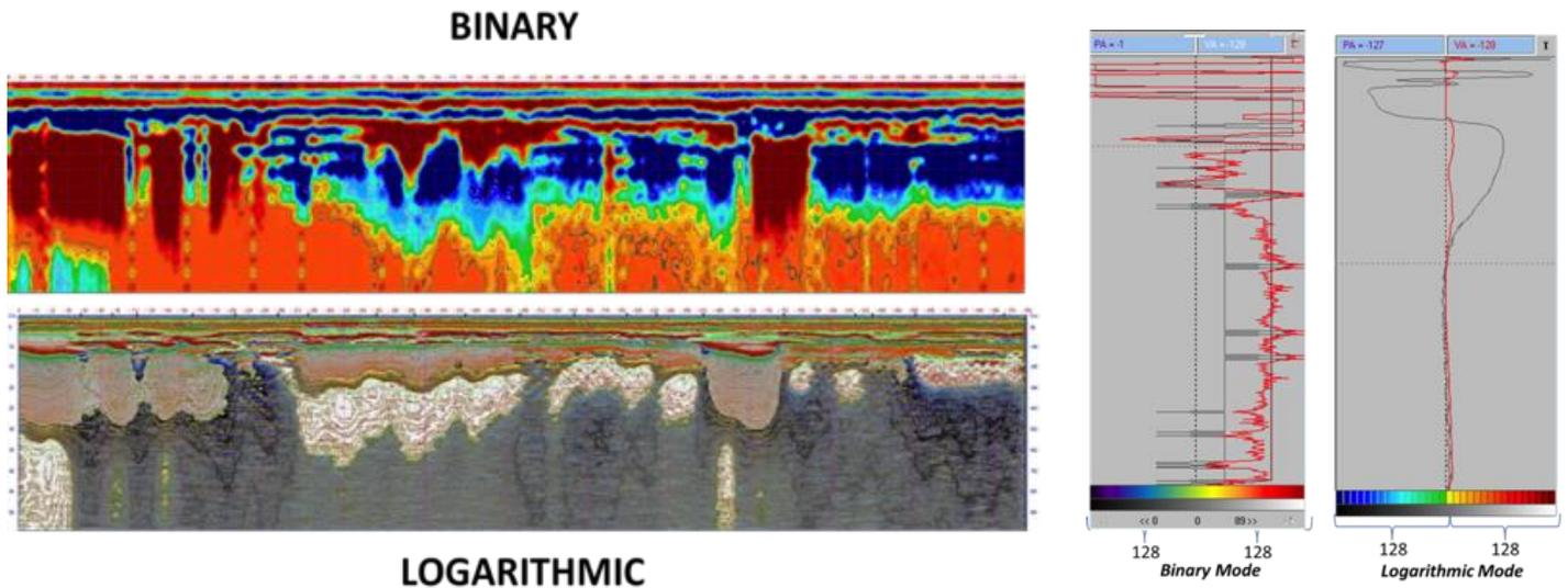
**Fig 2: Recording of the EM wave, showing different parameters - binary is a “quick method” using just one pulse of energy, Logarithmic uses many pulses to determine more detail.**
